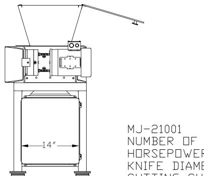
NUMBER OF MOTORS: 1 HORSEPOWER: 1HP ELECTRIC KNIFE DIAMETER: 4 3/4"
